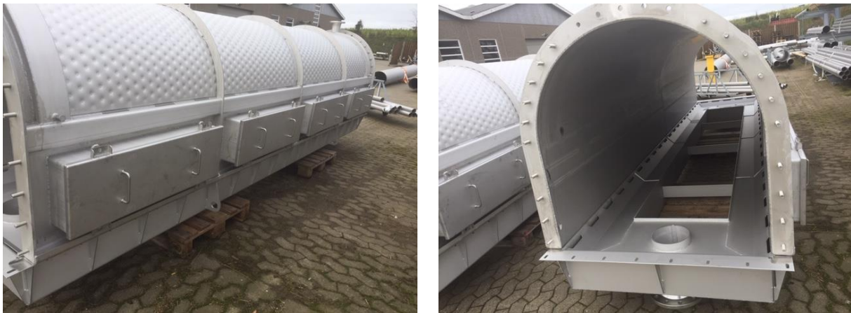
Figure 34: The jacket of the SHS-drier operates as MVR heat exchanger for the open loop heat pump. Picture is taken before mounting the SHS-drier.
