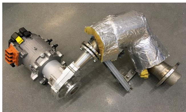
Figure 36: Flexible adjustment of the inlet and outlet of the EA42 unit enables standard connections (left), while the EC38 model needs a specially welded connection arrangement (right).
