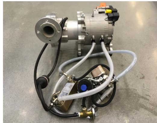
Figure 35: The two EA42 turbo-compressors from Rotrex mounted in the open loop heat pump (left). The cooling system requires only a water connection (top right) and not an external oil cooling system like the EC38 model (down right).
