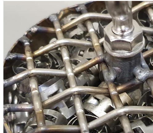
Figure 37: Bed of metal packings for improved and more compact de-superheating between compressor stage 1 and compressor stage 2.
