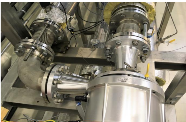
Figure 36: Flexible adjustment of the inlet and outlet of the EA42 unit enables standard connections (left), while the EC38 model needs a specially welded connection arrangement (right).
