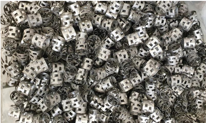
Figure 37: Bed of metal packings for improved and more compact de-superheating between compressor stage 1 and compressor stage 2.
