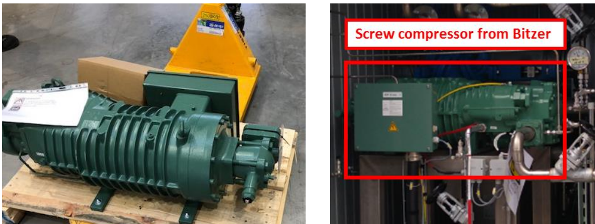
Figure 10: Bitzer compressor (left: before delivery; right: integrated in heat pump demonstrator)
