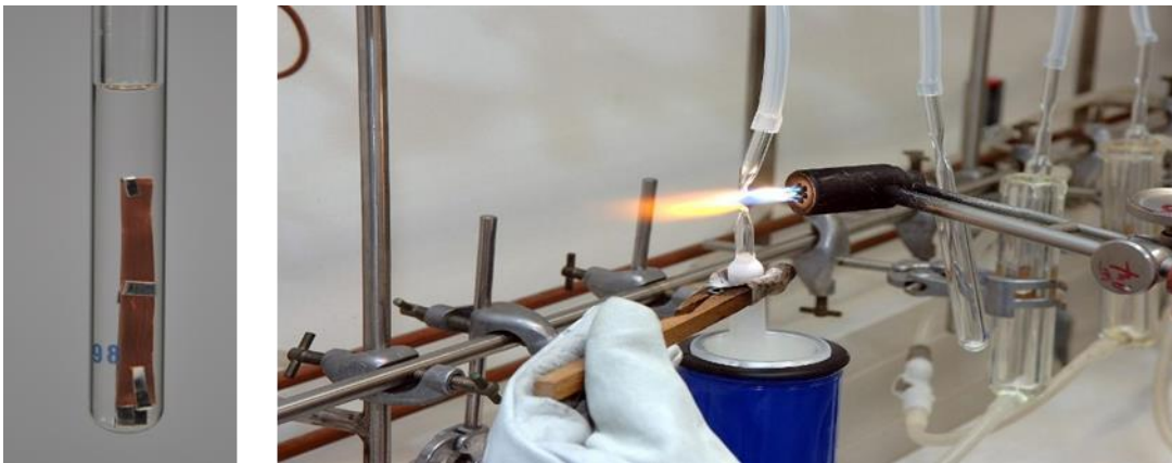
Figure 3: Preparation of sealed glass tubes for aging tests
