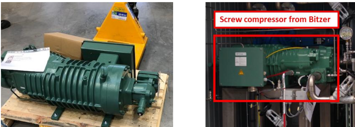
Figure 1: Bitzer compressor (left: compressor before delivery; right: integrated in heat pump demonstrator)
