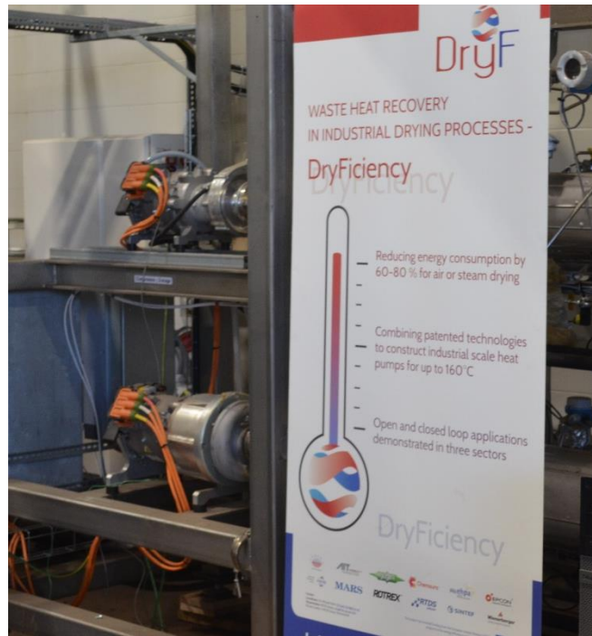
Figure 21: The two turbo-compressors of the open loop heat pump.
