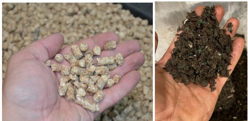
Figure 25: Dried fiber reject from food waste biogas plant (to the left) and final pellets from compost (to the right); both dried and processed with the SHS-drier of the pilot plant.
